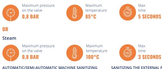
Before starting the filling sanitize the automatic/semiautomatic filling machine.
